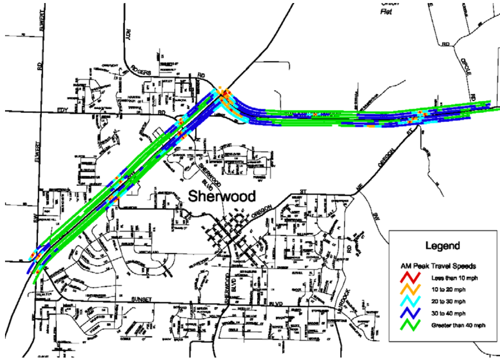
Figure 5 - Speed data recorded during multiple vehicle runs in as part of a study in Sherwood, Oregon.
